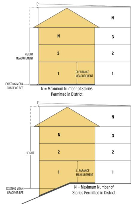
Figure 138-4421.f: BFE Less than or Equal to 2'
