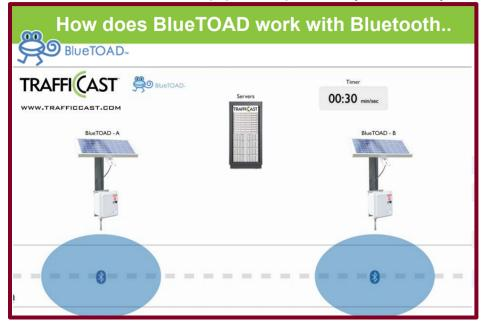
Bluetooth connections to the unique media access control addresses assigned to motorists' vehicles or mobile devices monitor and the progression of the vehicles corridors. through the Using this information, the BlueTOAD application calculates the average travel time for all motorists the corridor and on displays it on DMSs.
