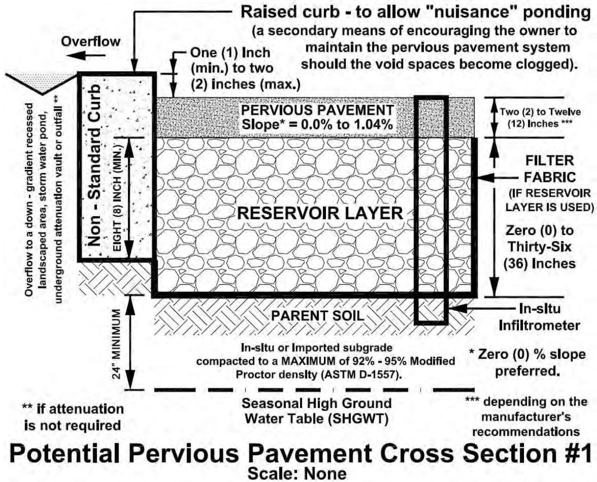
FIGURE 4.6.4. Pervious Pavement System Cross Section #1.
