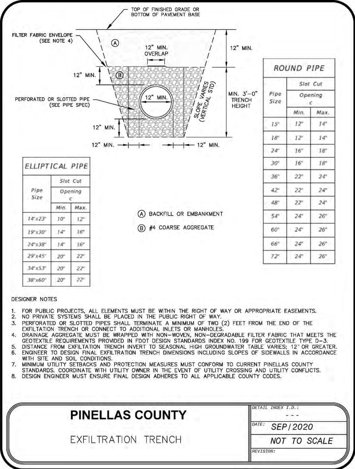
Figure 4.2.1: Pinellas County CAD template for exfiltration trenches
