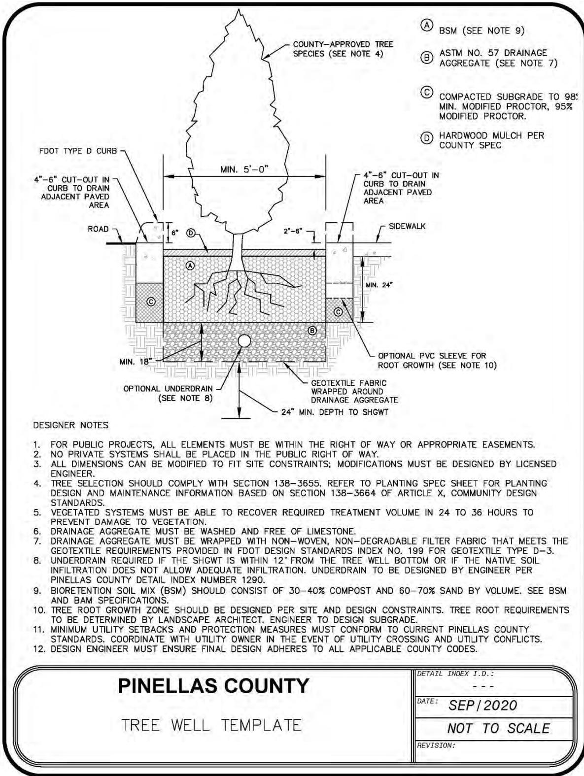
Figure 4.12.7: Pinellas County CAD template for tree wells
