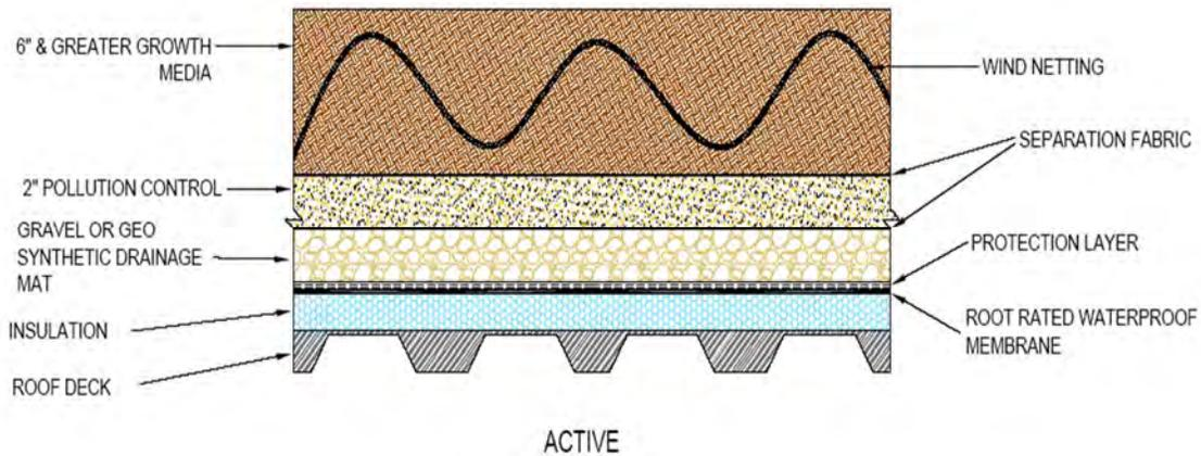
Figure 4.7.1b. Intensive Green roof Section (Usually Active Function)
