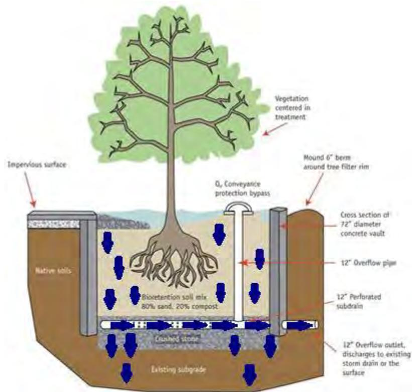
Figure 4.12 5. Example Stormwater Tree Box Filter System.
