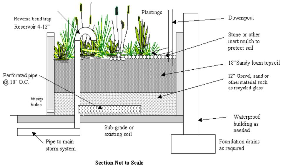
Figure 4.12.4. Example Stormwater Planter Box Biofiltration System.
