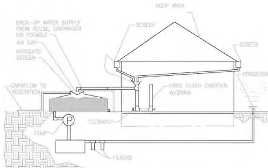
3. **Type 3 - Non-Potable System for Indoor and Outdoor Use with a Cistern** - The third type of system is a large residential or commercial system that stores rainwater in a cistern for indoor uses such as toilet flushing, urinal flushing, HVAC make-up water, laundry wash water, and other outdoor uses. In these systems:
