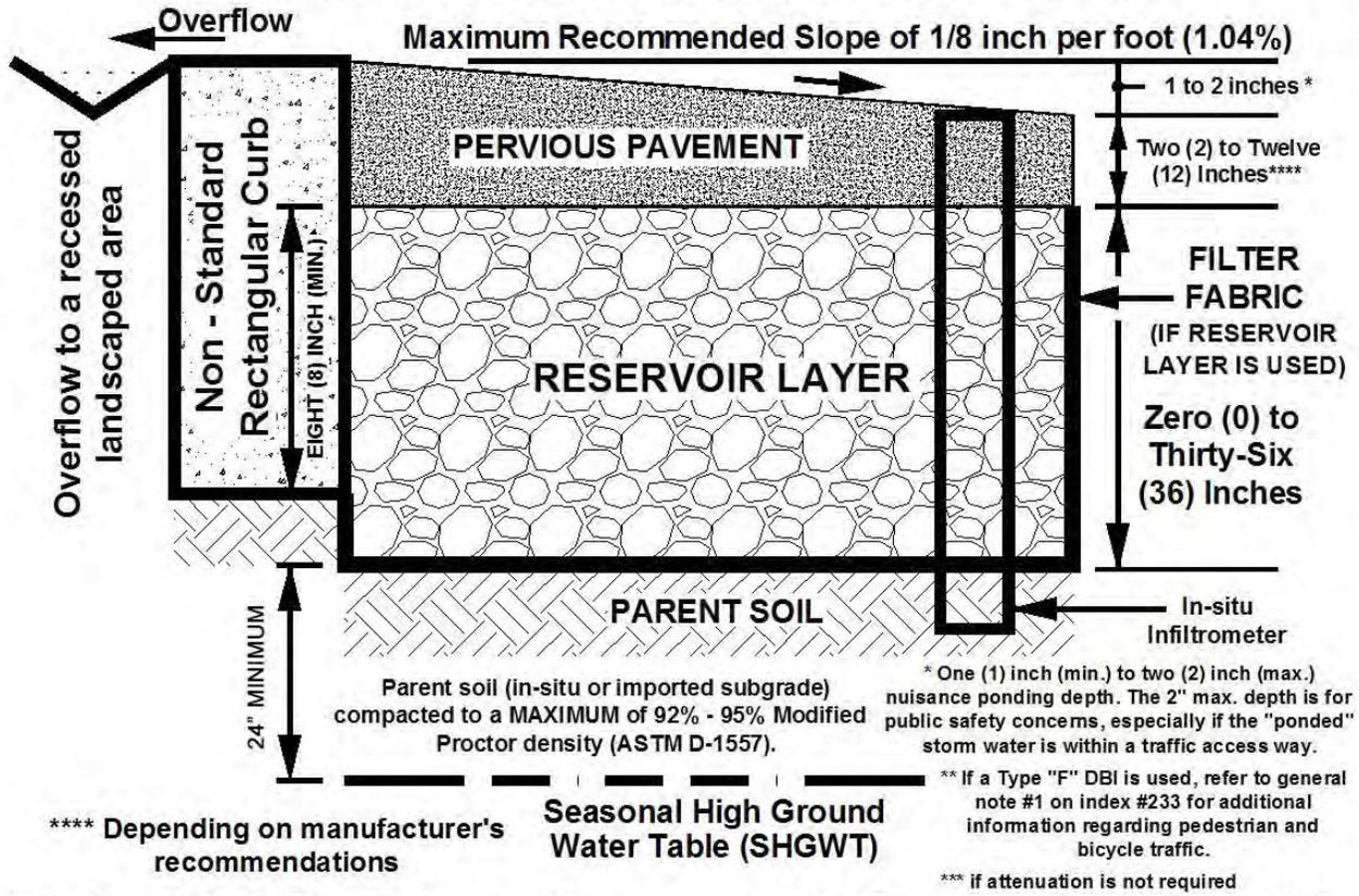
**Potential Pervious Pavement Cross Section #3**
