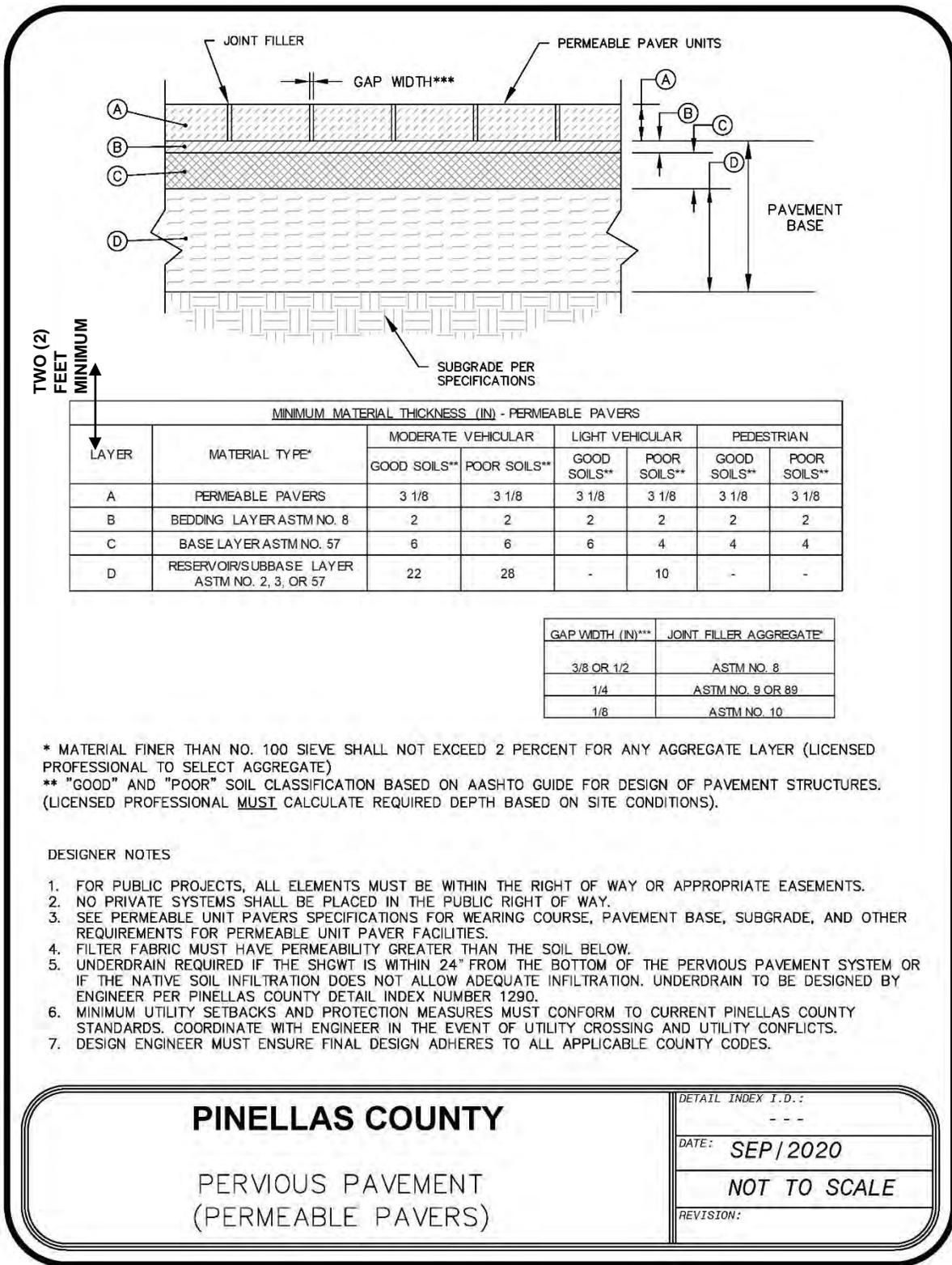
\* MATERIAL FINER THAN NO. 100 SIEVE SHALL NOT EXCEED 2 PERCENT FOR ANY AGGREGATE LAYER (LICENSED PROFESSIONAL TO SELECT AGGREGATE)
