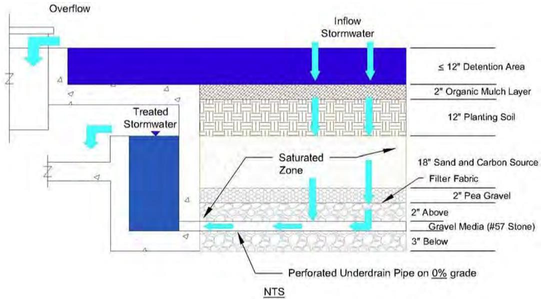
Figure 4.12.3. Cross Section View of System with Overflow.
