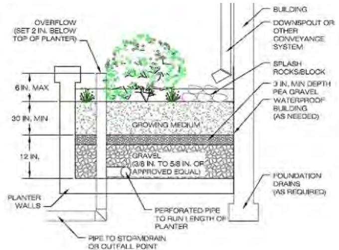
5. **Liners** - Flow-through facilities that require an impervious bottom can be achieved through either a waterproof liner (geomembrane) or a single-pour concrete box. If lined, there are many liner options, and installation varies. Liners should be installed to the high water mark. Liner will be 30 to 40- mil PVC or HDPE as appropriate or approved equivalent.
