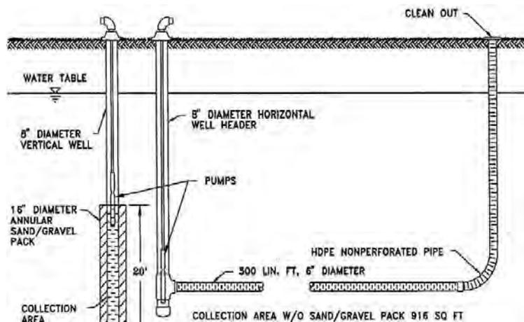
Figure 4.9.3. Example Schematic for Stormwater Harvesting Withdrawal System.
