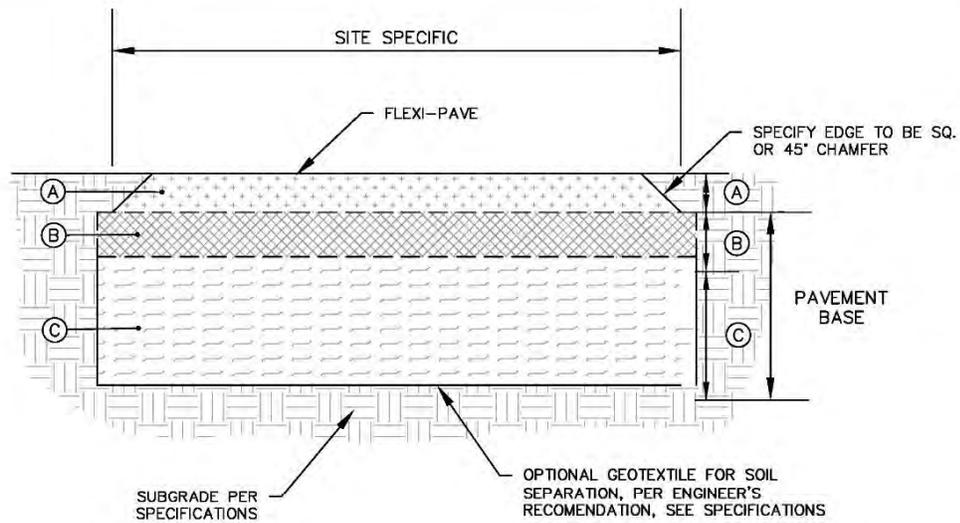
**MINIMUM MATERIAL THICKNESS (IN) - FLEXI-PAVE**
