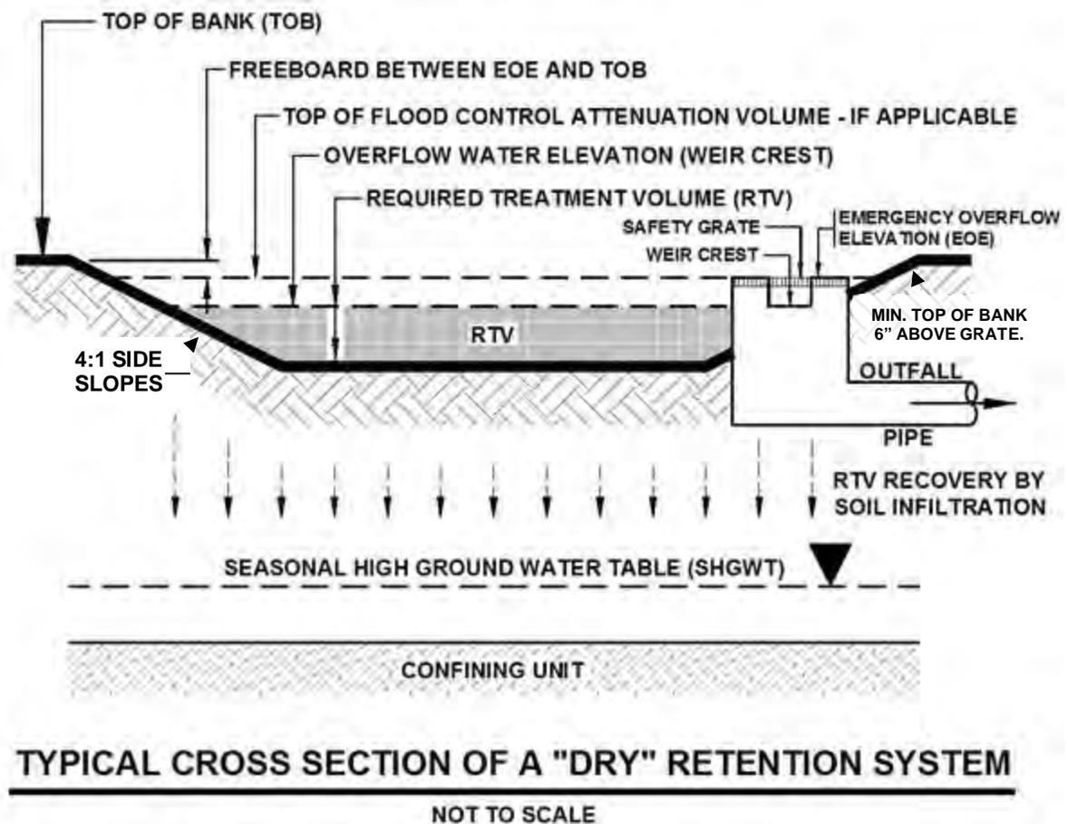
Figure 4.1.1. Typical Cross-section of "Dry" Retention Basin
