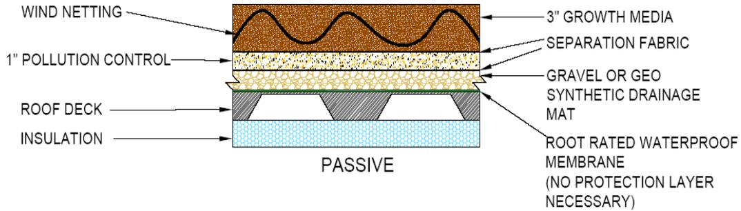
Figure 4.7.1a. Extensive Green roof Section (Usually Passive Function)
