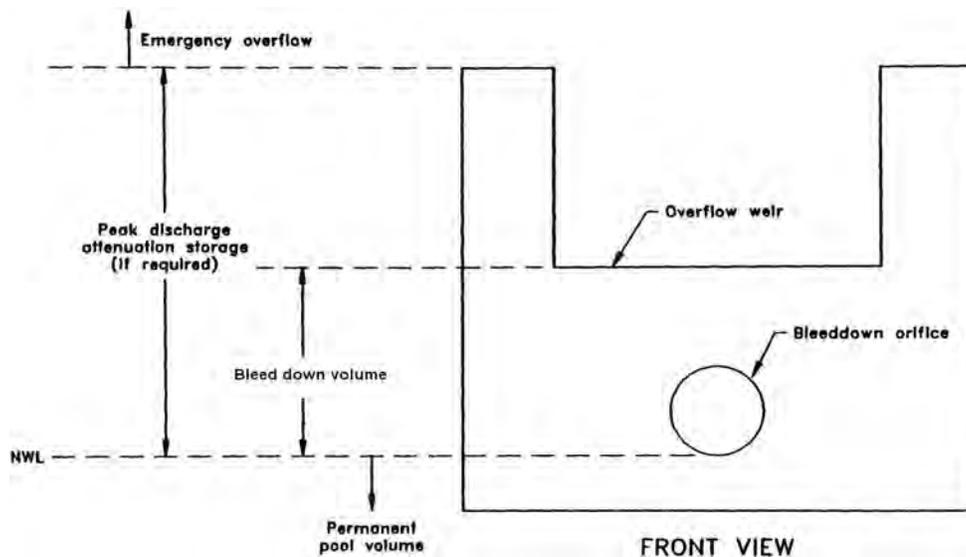
Figure 4.8.4. Typical Wet Detention Outfall Structure (N.T.S.).
