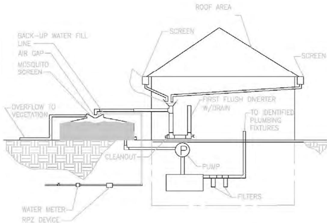
4. **Type 4 - Potable Use with a Cistern** - The fourth type of system is a residential or commercial system that stores rainwater in a cistern as a source of potable water. This type of system is designed for human consumption. Therefore, the system has additional design, operating, and permitting requirements from the [Pinellas County Health Department](#).
