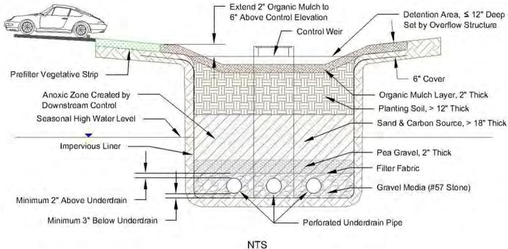
Figure 4.12.2. Cross Section View of a Biofiltration System.
