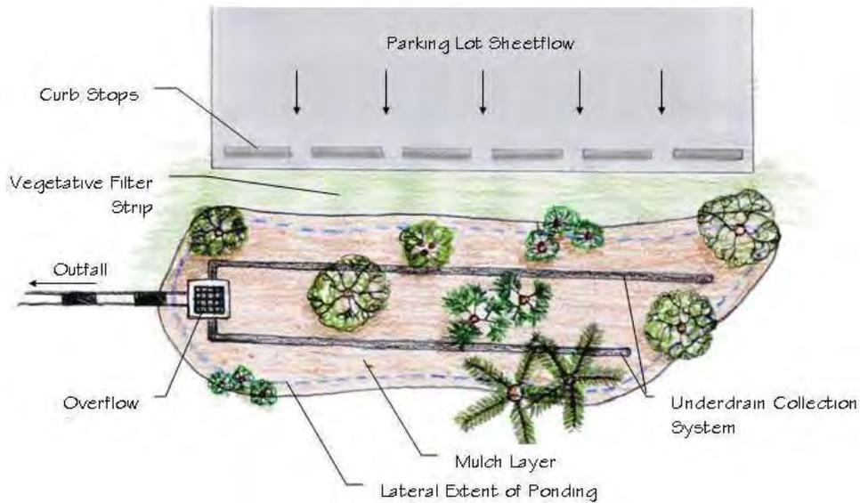
Figure 4.12.1. Plan View Illustrating a Biofiltration System.
