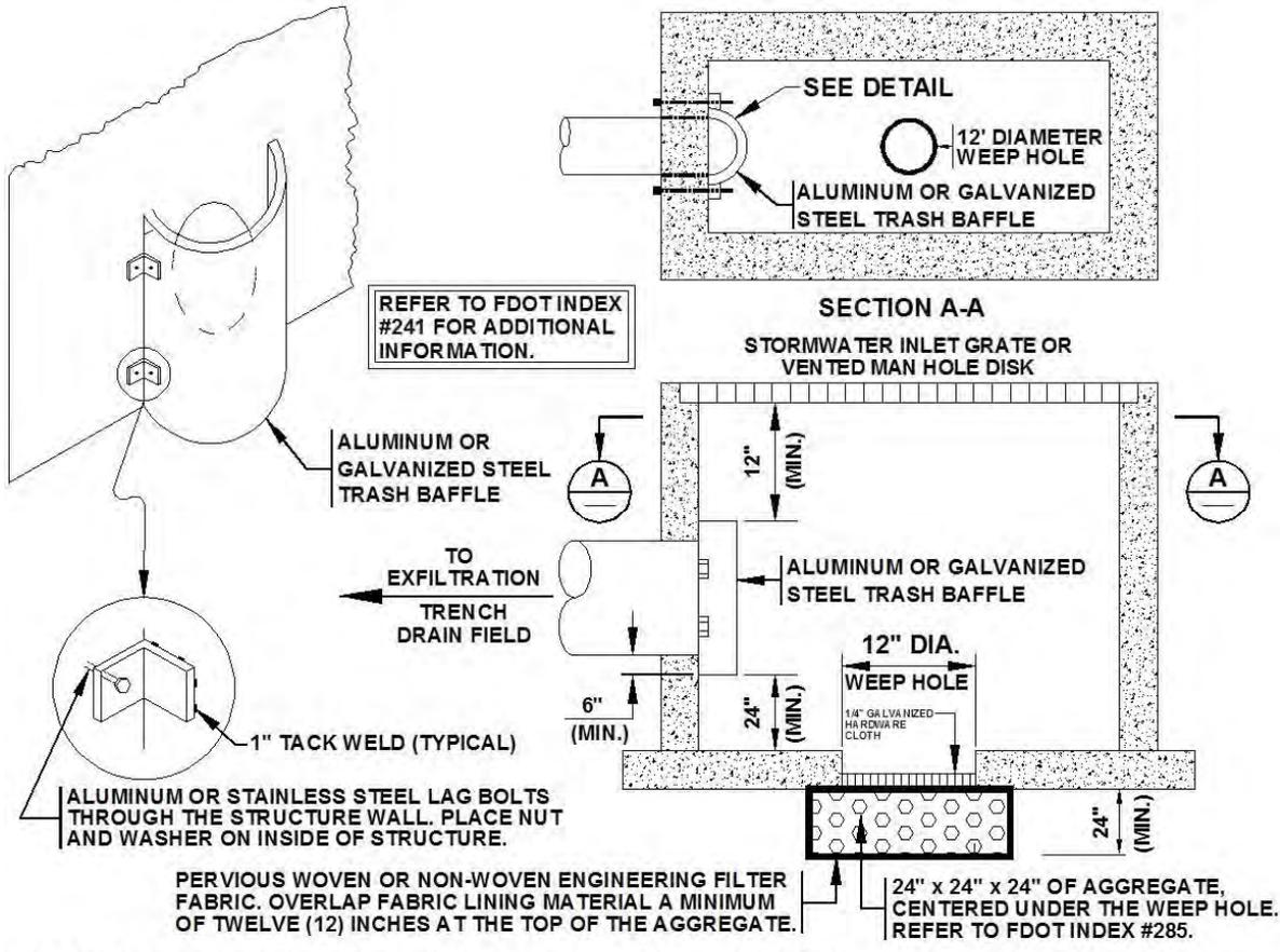
**"GENERIC" DETAIL FOR AN EXFILTRATION TRENCH SEDIMENT / TRASH BAFFLE**
