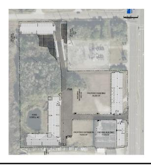
**Summary:** ESP application 45390, Racetrack430 LLC, plans to rehabilitate an existing 23,410 square foot industrial building with a 19,453 square foot addition and construct an additional 50,000 square foot freestanding building on the site. Along with the new industrial square footage will be additional parking, potable water upgrades, a fire suppression system, stormwater upgrades and a private sanitary sewer lift station.
