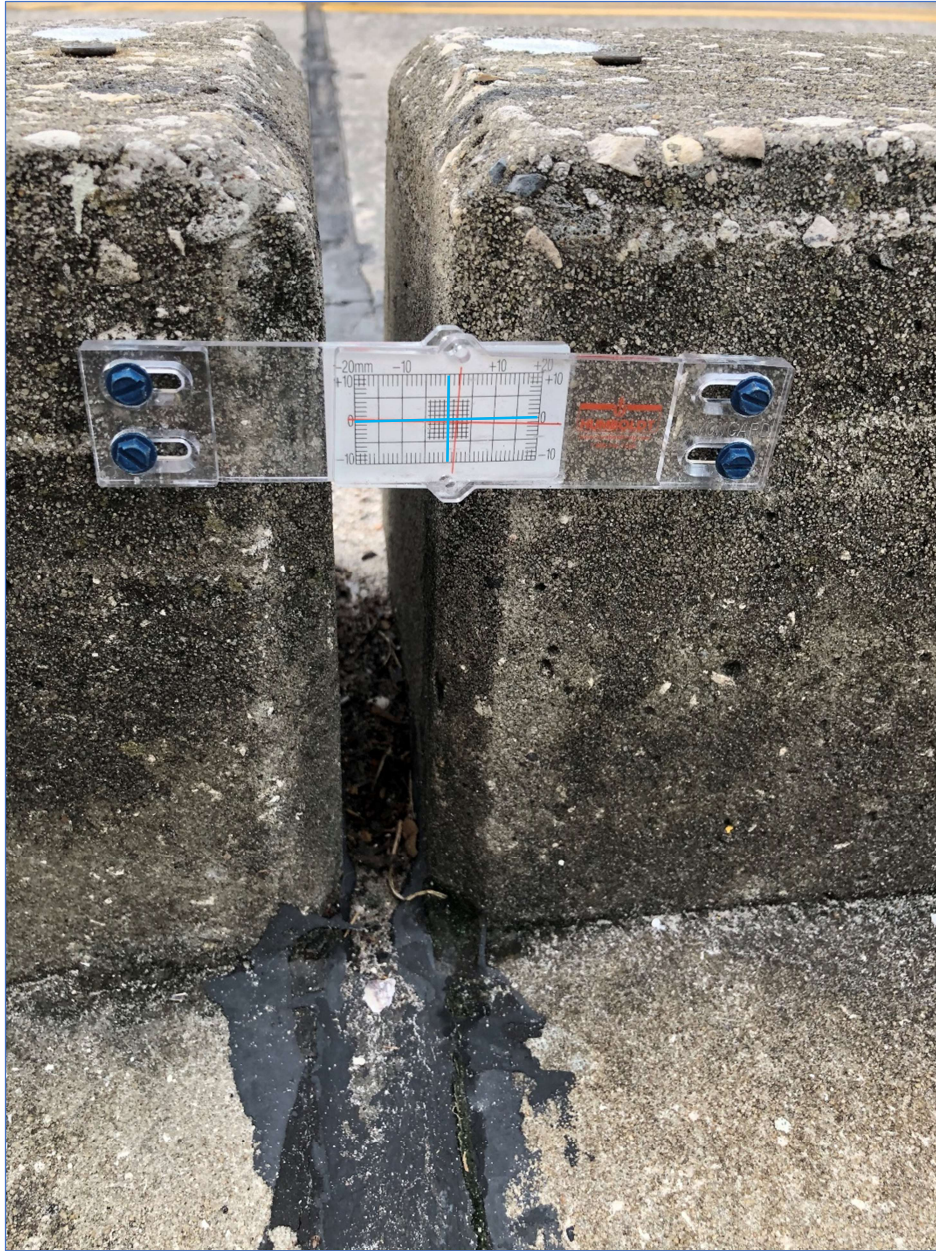
Photo 11 - Monitoring Devices at Face of Curb with Evidence of Settlement/Rotation
