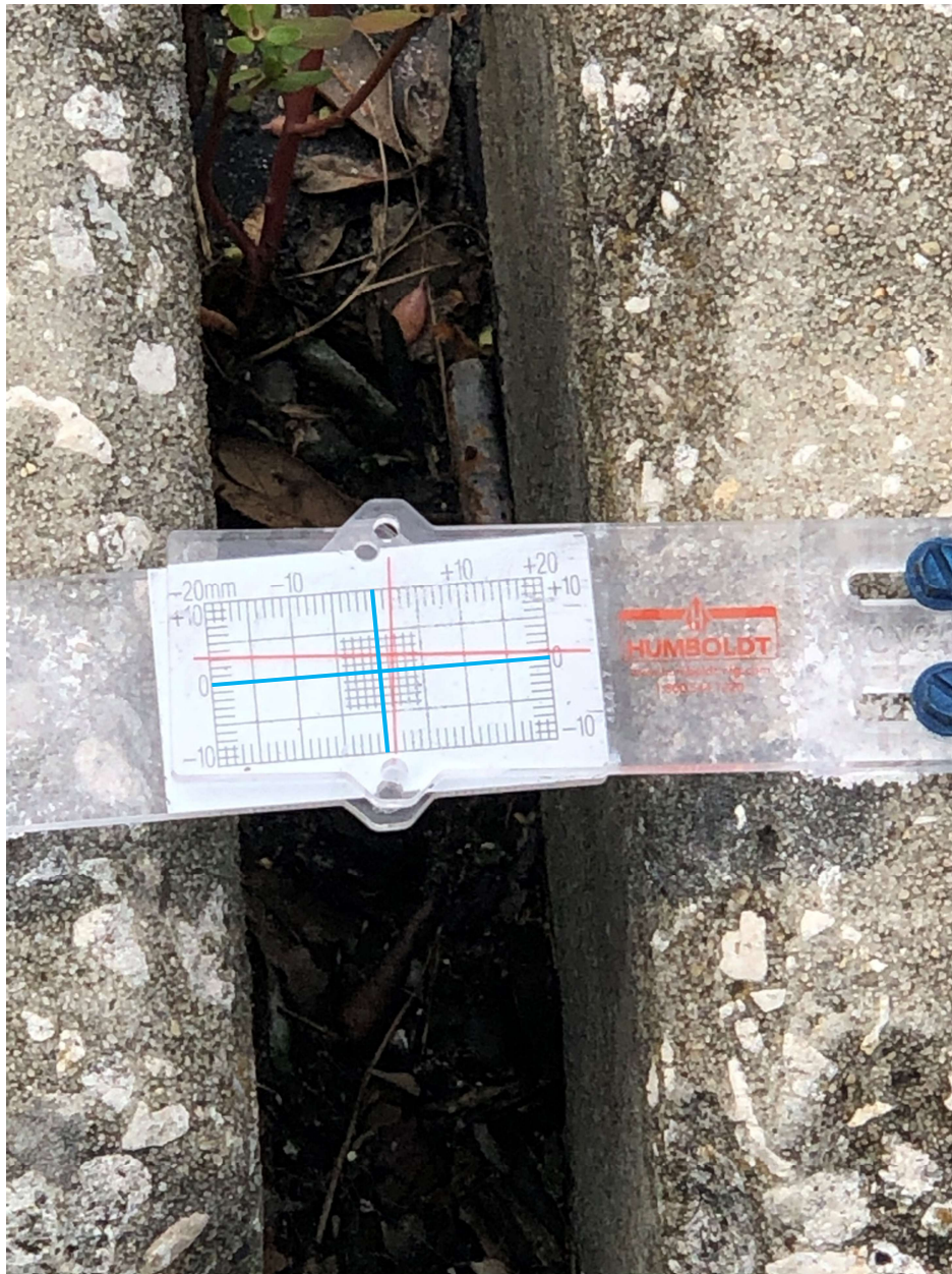
Photo 10 - Monitoring Devices on Top of Curb with Evidence of Lateral Movement/Rotation
