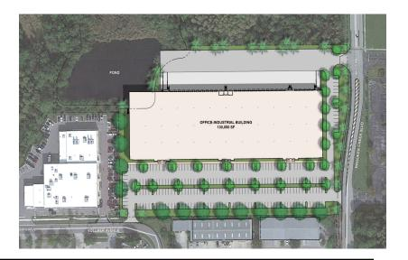
**Summary**: ESP application 45245, Brooker Creek V LLC, is an industrial new construction project that proposes a 130,000-square-foot single story, 30' clear height ceiling that will be tilt-wall constructed and located in the City of Oldsmar. If provided ESP funding, the developer anticipates it will take 264 days to build the project.
