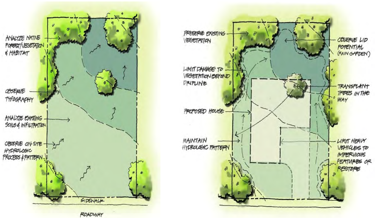
Figure 6.7.1. Site Planning responding to existing conditions.
