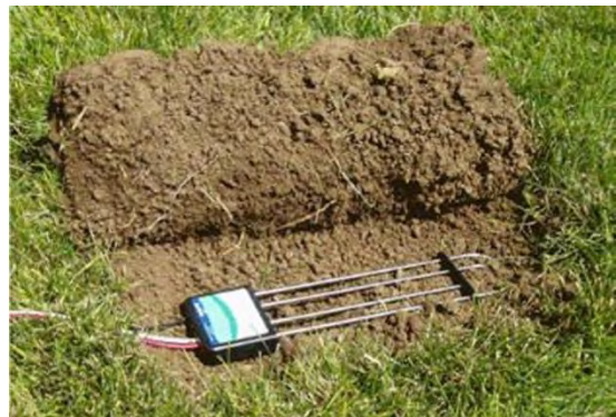
A soil moisture sensor, buried in the turf root zone prevents irrigation when it is not needed.
