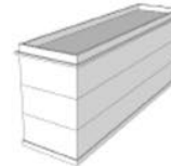
Flat or shed roof behind parapet
