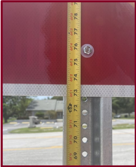
Figure 1 - Stop sign height does not meet requirements (seven feet)
