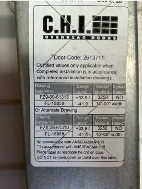
Site 2: Park Buildings, 6 each of C.H.I./3250/Ribbed Steel C.H.I. Overhead Coiling Doors, 10 FT long x 10 FT high, 3 feet of surge water pressure pushed the doors inward into the building., 100% work completed.
