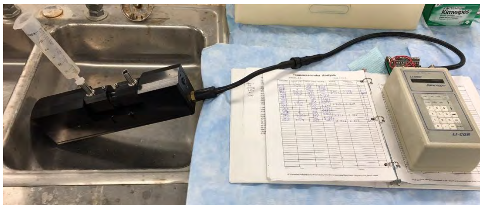
Figure 3: Complete set-up for taking transmissometer readings (05-22-17).
