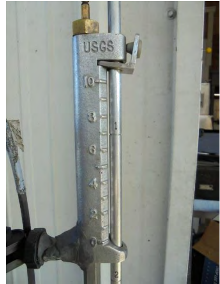
Figure 5c and d. Example of how to set rod to measure velocity at 60% of 0.6 feet total depth, and for 1.7 feet total depth.
