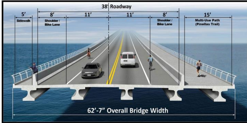
Figure 3. Preferred Alternative Bridge Section
