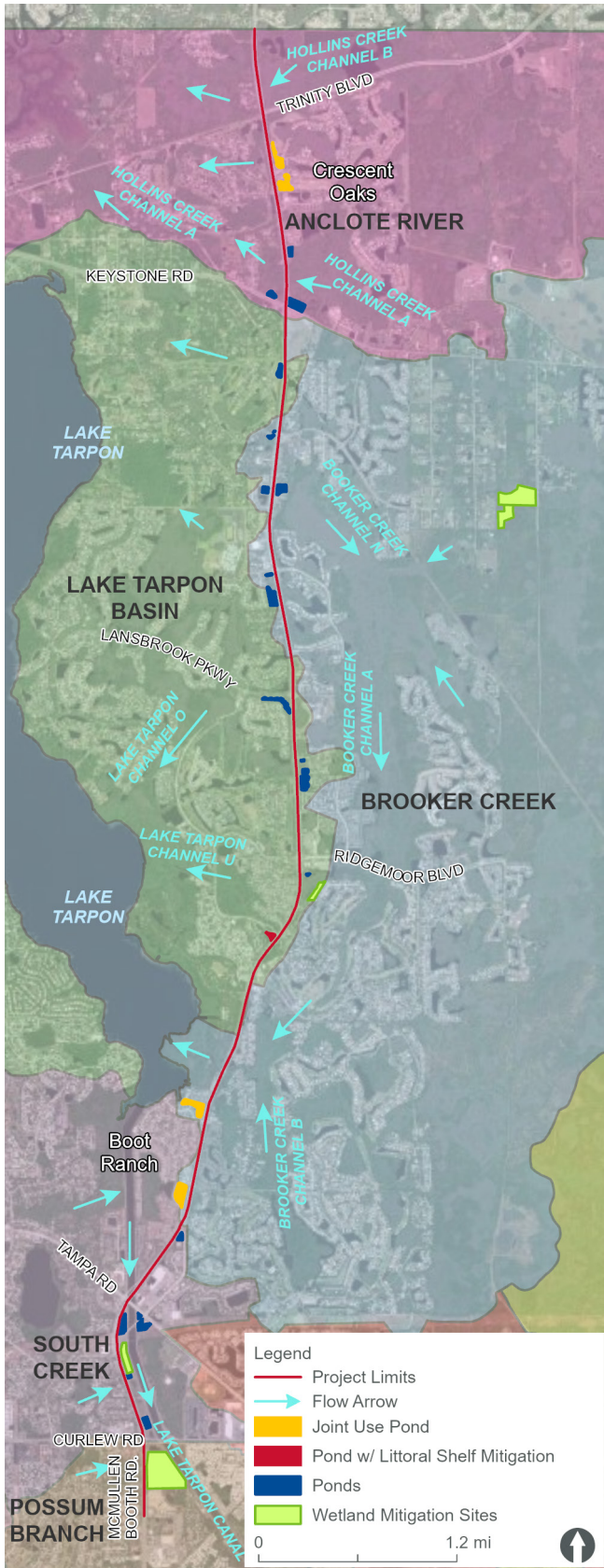
Figure D-1: Existing Stormwater Management Exhibit
