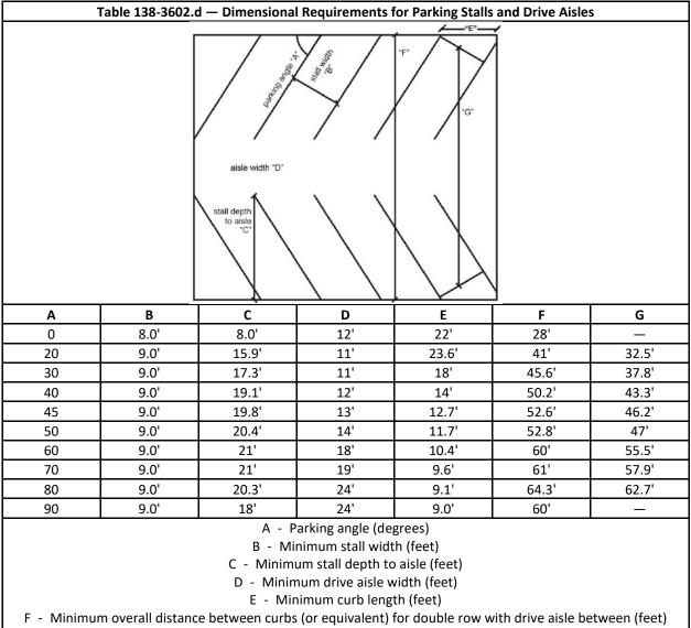
G - Minimum distance between ends of stalls (or equivalent) for double row with drive aisle between
