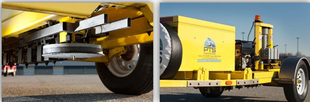
Photos of PTS's Dynatest Model 8000 FWD
