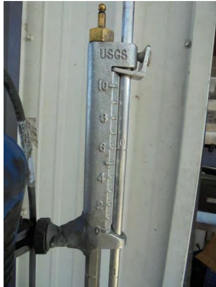
Figure 5c and d. Example of how to set rod to measure velocity at 60% of 0.6 feet total depth, and for 1.7 feet total depth.
