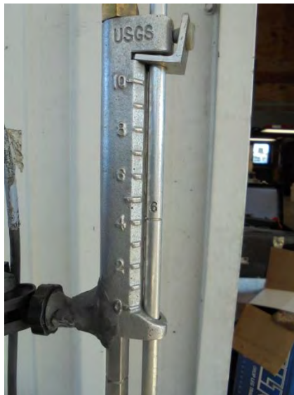
Figure 6a and b. Example of how to set rod to measure velocity at 20% and 80% for 3.2 feet total depth.
