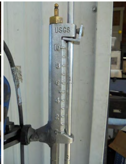
Figure 6a and b. Example of how to set rod to measure velocity at 20% and 80% for 3.2 feet total depth.
