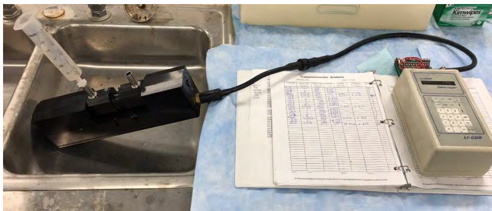
Figure 3: Complete set-up for taking transmissometer readings (05-22-17).
