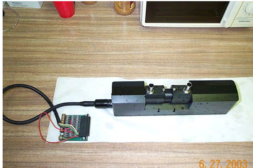
Figure 2: Transmissometer with pig-tail and wire-block assembly attached and 10-cm flow-through cell in place.
