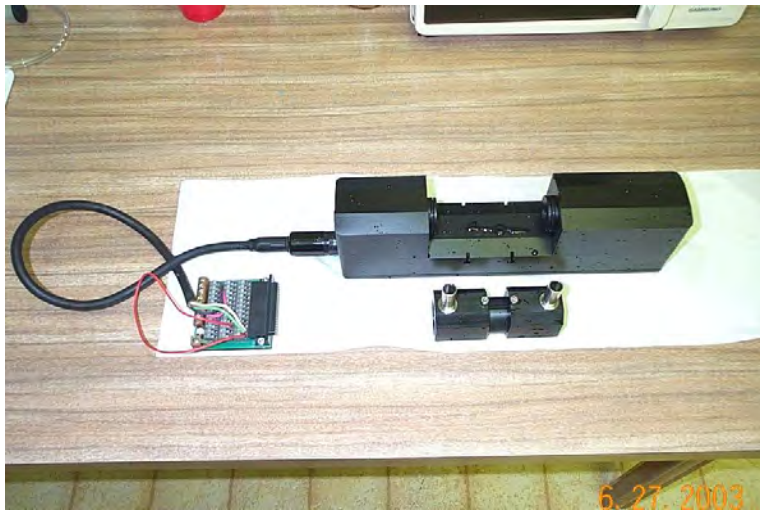
Figure 1A: Transmissometer with pig-tail/wire-block assembly already attached and 10-cm flow-through cell not in place.
