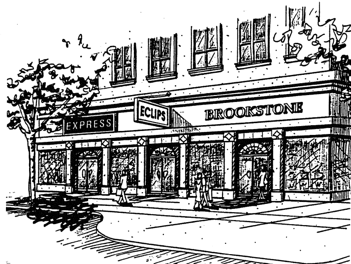
Various Sign Installation Formats within a Facade - Unacceptable
