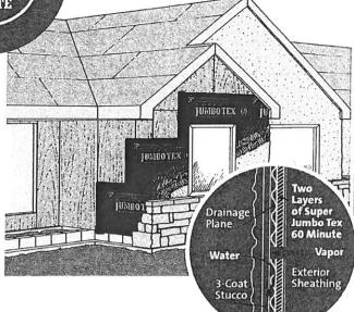
Super Jumbo Tex 60 Minute protects against water intrusion from the outside, while allowing moisture to escape from the inside.
