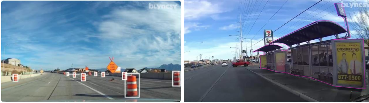
Figure PS-12. Automated Detection of Work Zones and Bus Stops
