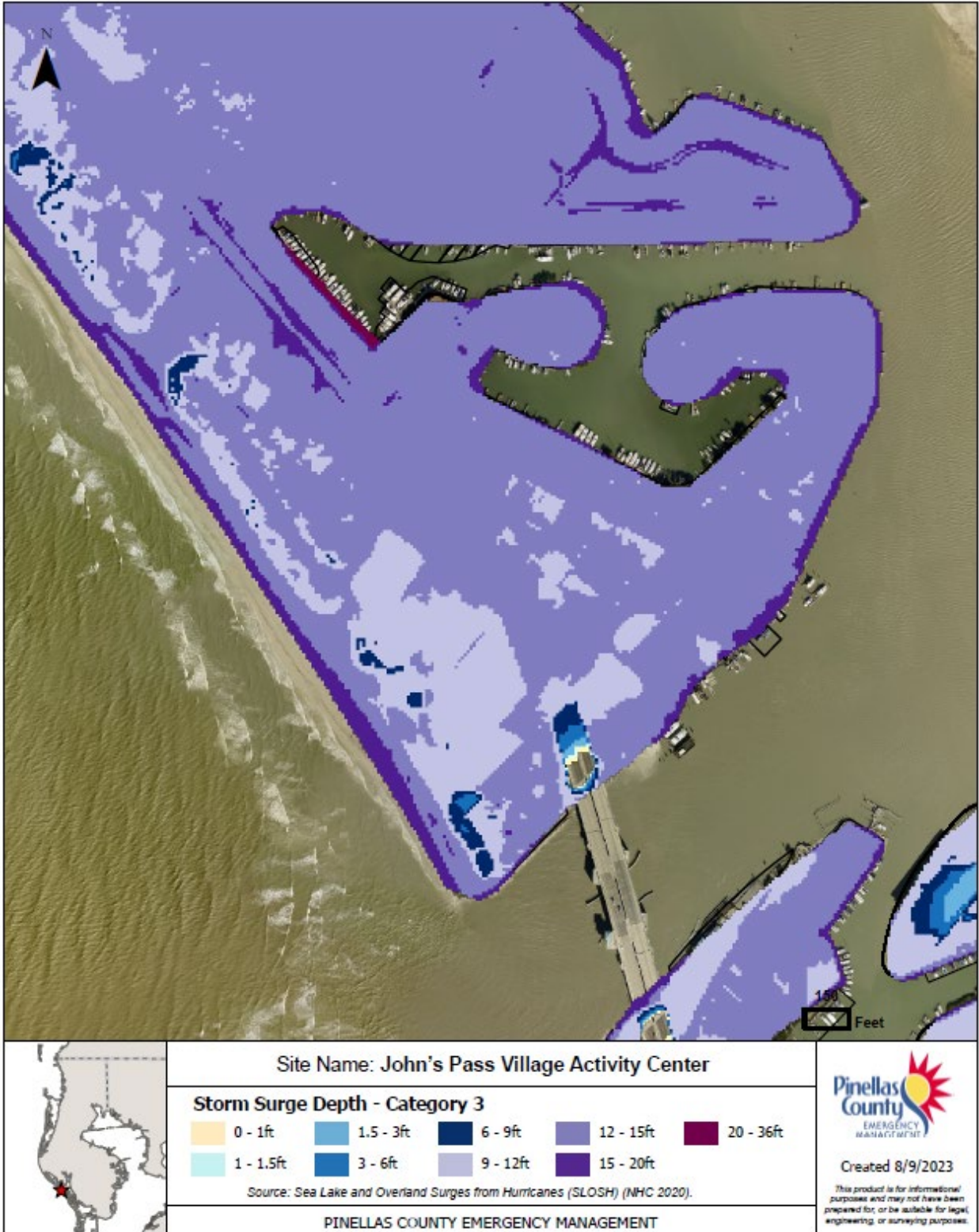
Attachment 7. Category 3 surge inundation depth (ft). Source: NHC SLOSH Model, v2020.
