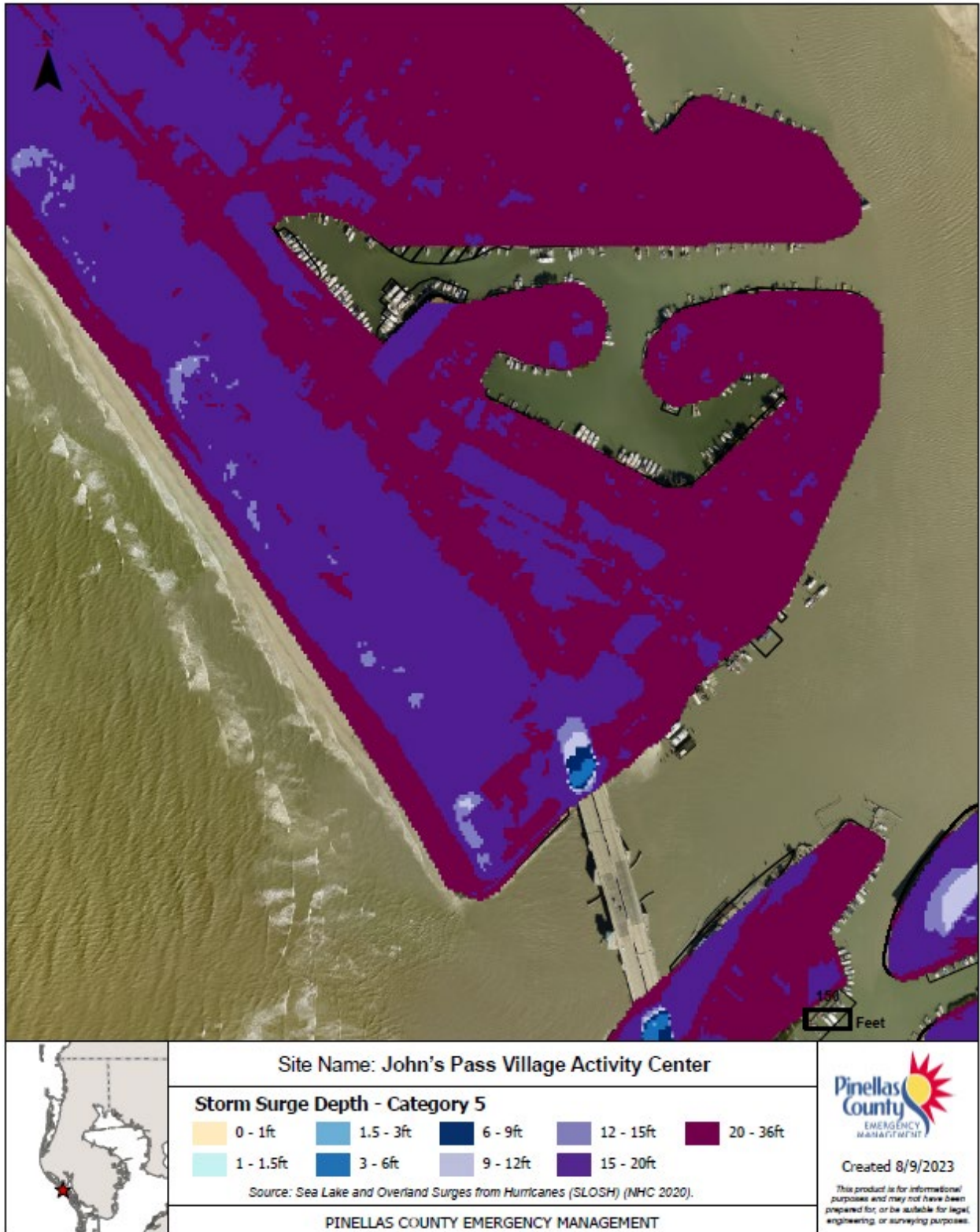
Attachment 9. Category 5 surge inundation depth (ft). Source: NHC SLOSH Model, v2020.
